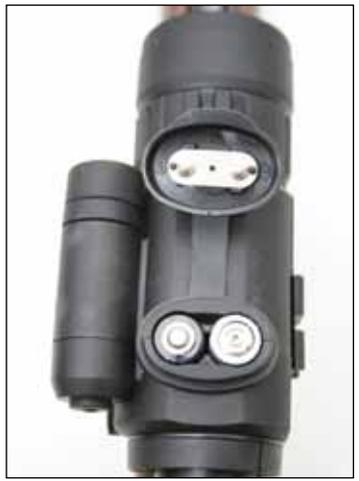
Two AA batteries held vertically to stop recoil bounce disconnecting them
